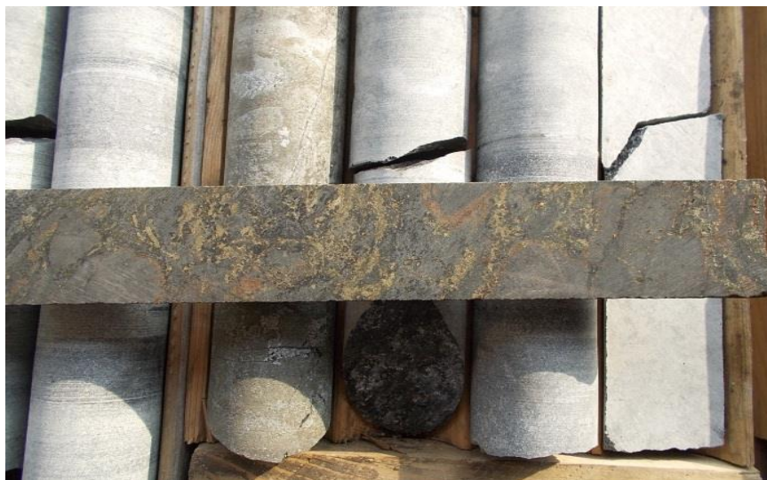
Wabassi “E” Deposit, hole 11WA-16 showing rhyolite breccia with sulphide matrix (“Mill Rock”)
