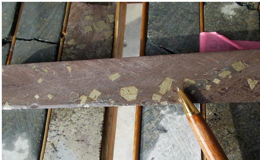
Wabassi “E” Deposit, hole 11WA-16 showing massive zinc mineralization ( red-brown sphalerite) with recrystallized pyrite crystals
