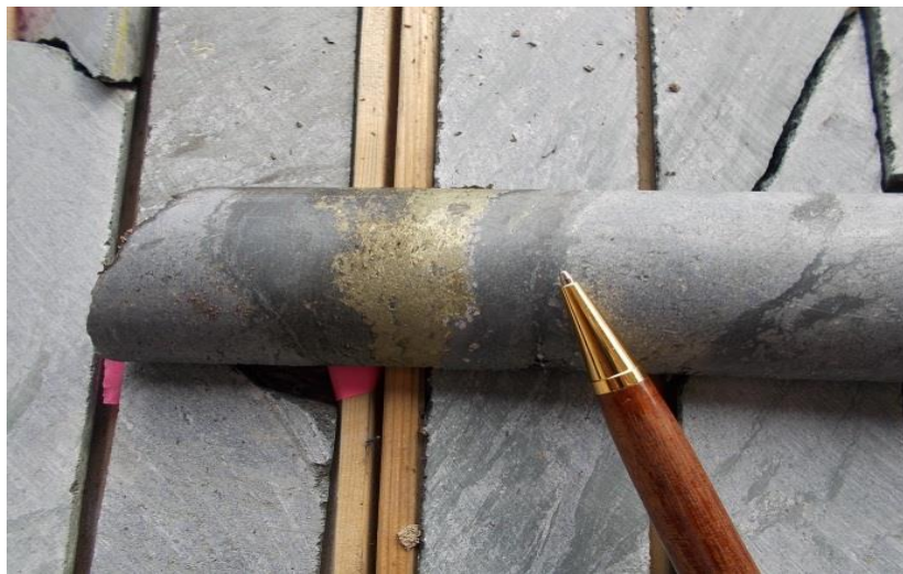
Wabassi “E” Deposit, hole 12WA-28 showing stringer Cu mineralization (chalcopyrite) associated with chlorite vein alteration
