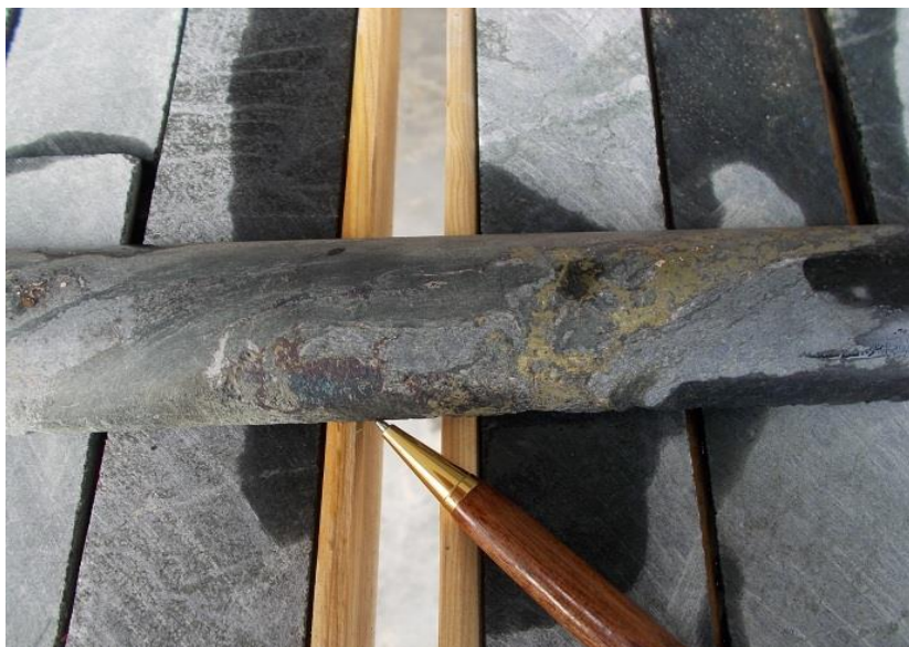
Wabassi “E” Deposit, hole 12WA-28 showing stringer Cu mineralization with chalcopyrite and bornite (at pen) with chlorite alteration
